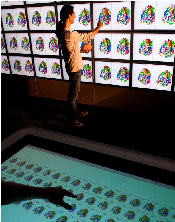
Figure 1: Multi-surface interaction with the BrainWall: multiple users interact with a table, wall-sized display, and physical interface props.
